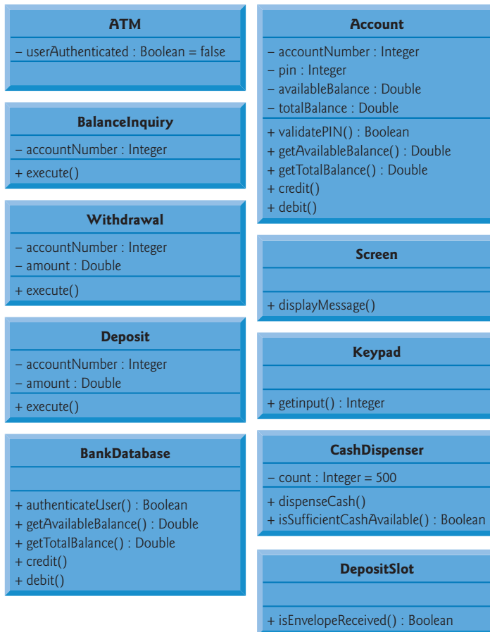
Fig. 26.1 | Class diagram with visibility markers.
